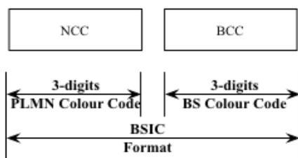
**Figure 6: GSMA Spec. 03.03 Format for BSIC**
