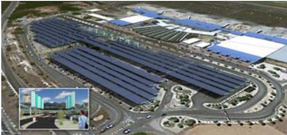
Aruba Airport: impression of the USD 11 mln. solar covered parking project, with charging stations for electric cars. It will generate 3 MW, equivalent to the power the airport uses during its peak hours, to be completed by the end of 2014.
